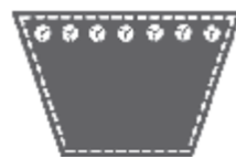
optibelt VB S=C Plus in cross section
